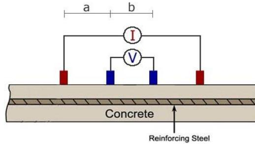
**Figure 1.** The configuration of 4 probes on the surface of concrete for corrosion detection of rebar inside the concrete
