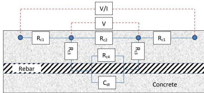
**Figure 3.** Electrical circuit of reinforced concrete system in non-contact four-probe measurement
