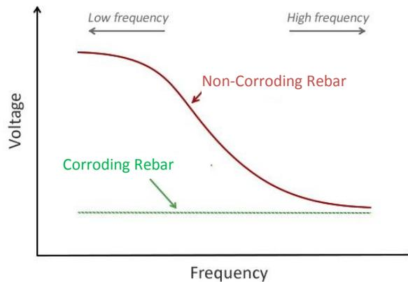
**Figure 2.** The schematic illustration of the voltage-frequency response of the corroding rebar compared to the non-corroding rebar
